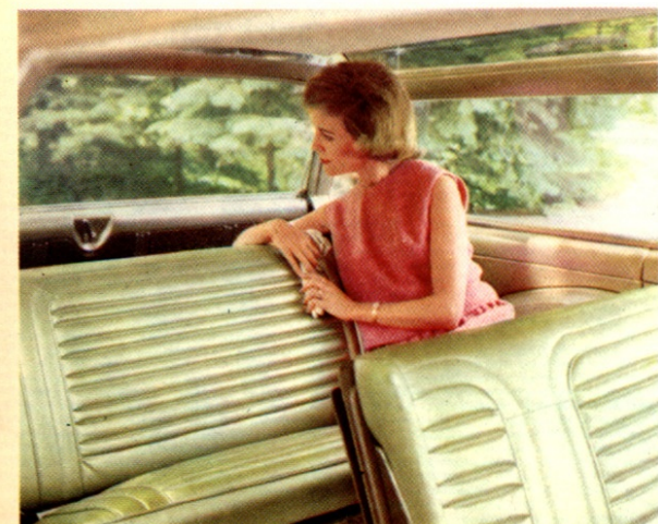
Vista-Cruiser's third seat faces forward, folds down easily to accommodate cargo. All-Moroccan or Moroccan-and-cloth interiors are as neat and pretty as they are practical!
