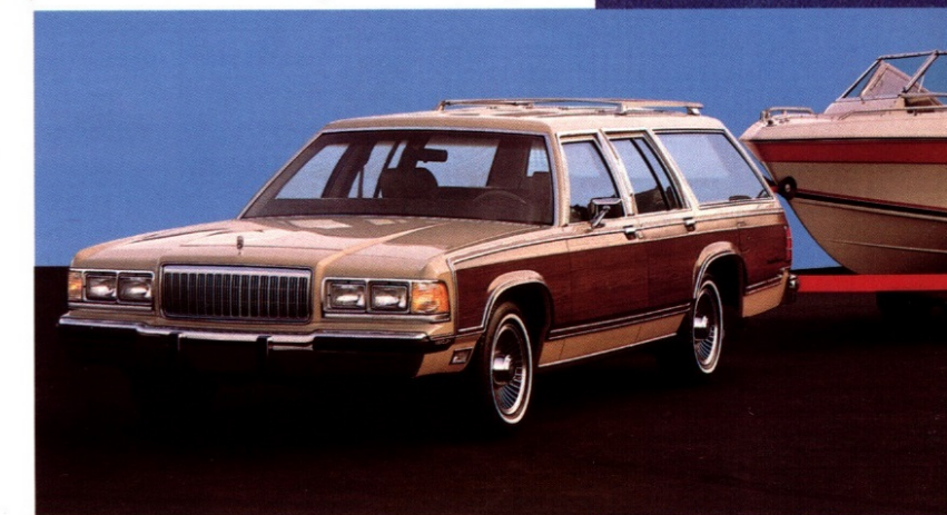
Trailer towing is easy with Grand Marquis' optional trailer towing package. It allows Grand Marquis sedans and Colony Park wagons to tow up to 2268 kg (5,000 lb.), (2721 kg (6,000 lb.) with the optional 5.8 L V-8 engine/2.73:1 axle ratio).
