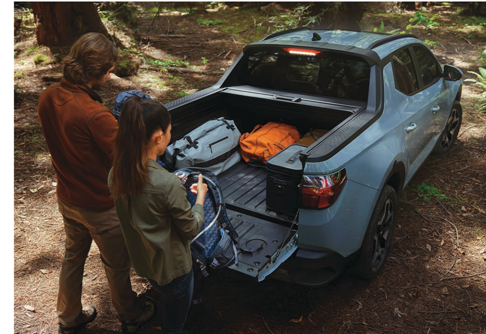
Sheet molded composite bed with rail system, adjustable tie-down cleats and LED bed lighting
