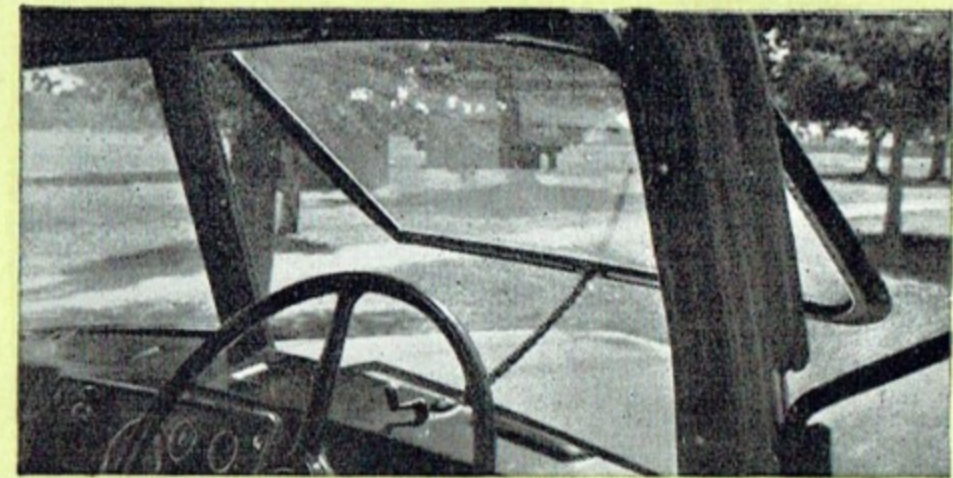
The driver's windscreen opens and can be adjusted as desired to provide extra cab ventilation.
