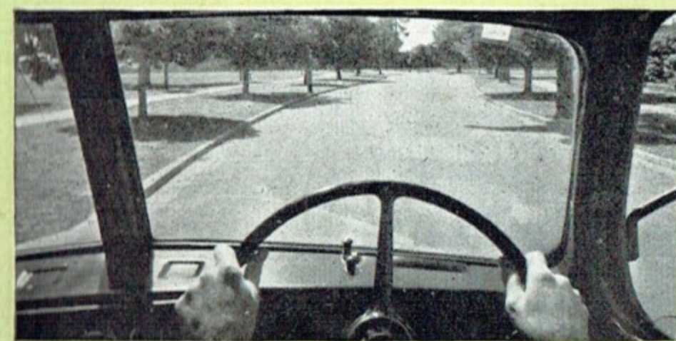
The windscreen is designed in a semi-V shape to deflect glare. Broad windows give maximum visibility.
