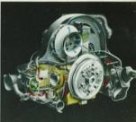
4-cylinder, 4-stroke, O.H.V. type VW engine, rear-Engine
