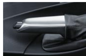
Leather-covered handbrake grip with decorative strip in chrome For Saloon and Touring.
