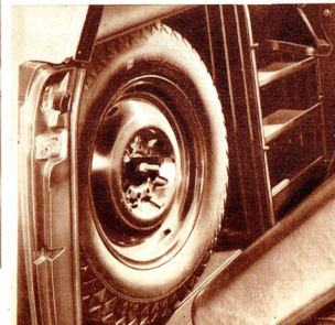
A convenient space for the spare tire of coupes is provided behind the seat. Also notice the roomy package shelves.
