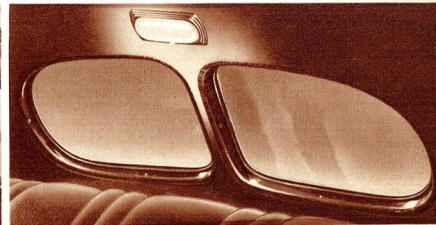
The dome light, just above the divided rear window, is a real reading light for rear seat passengers. The switch is on the center door pillar, curb side, for convenience at night.
