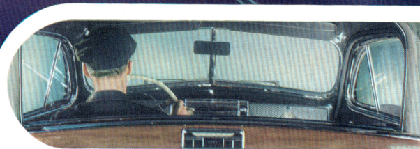
The sliding glass partition between the driver and passenger compartments may be raised as far as desired or lowered entirely simply by pressing a button control in the rear-seat armrest.
