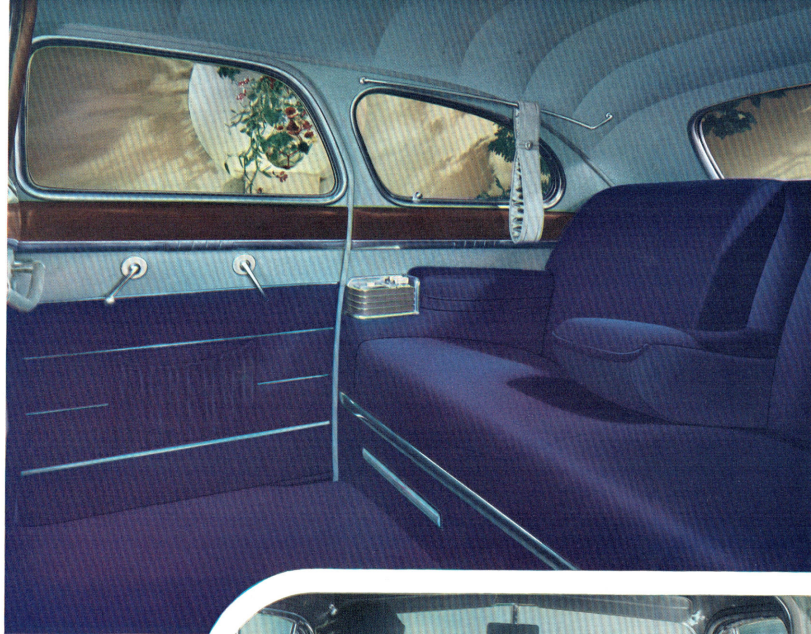
The sliding glass partition between the driver and passenger compartments may be raised as far as desired or lowered entirely simply by pressing a button control in the rear-seat armrest.
