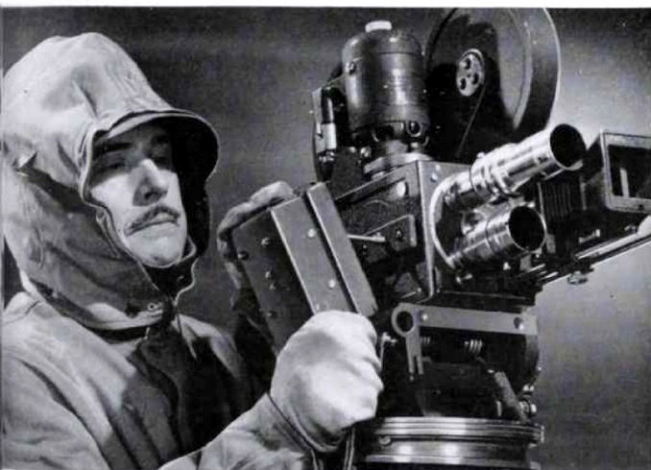
CAMERA HEATER. Heating device developed by Studebaker enables motion picture cameras to operate in coldest weather.
