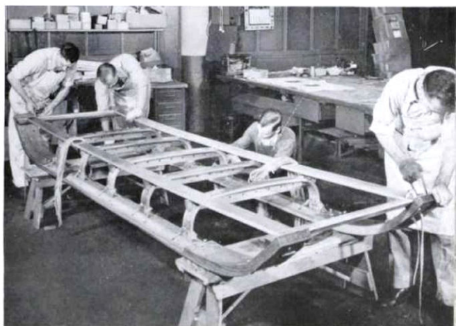
SLEDS. For use over snow terrain, wooden sleds are built for the Army. Parts are lashed together with rawhide.
