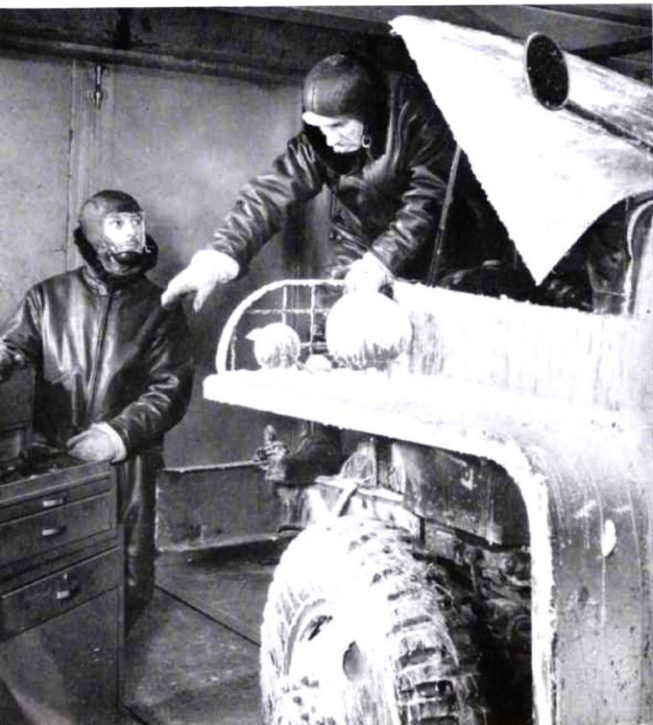
COLD ROOM. Temperatures 60 to 70 degrees below zero reveal how trucks will behave in Arctic cold.
