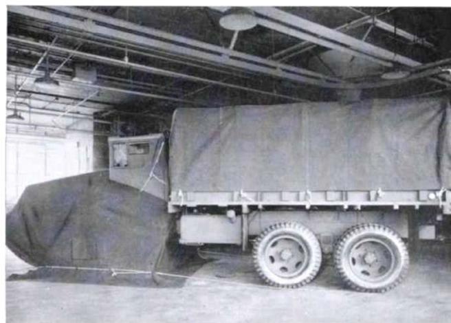
ENGINE HEATER. This heating installation permits engines to start promptly in severe cold weather.
