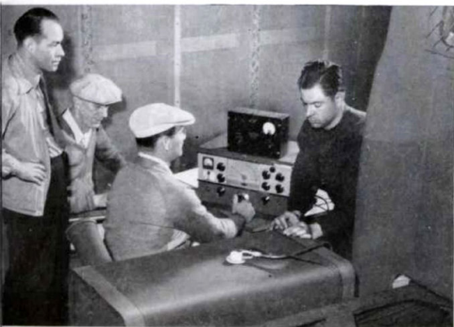
RADIO INTERFERENCE SUPPRESSION. In special rooms, trucks are checked for interferences affecting radio installations.
