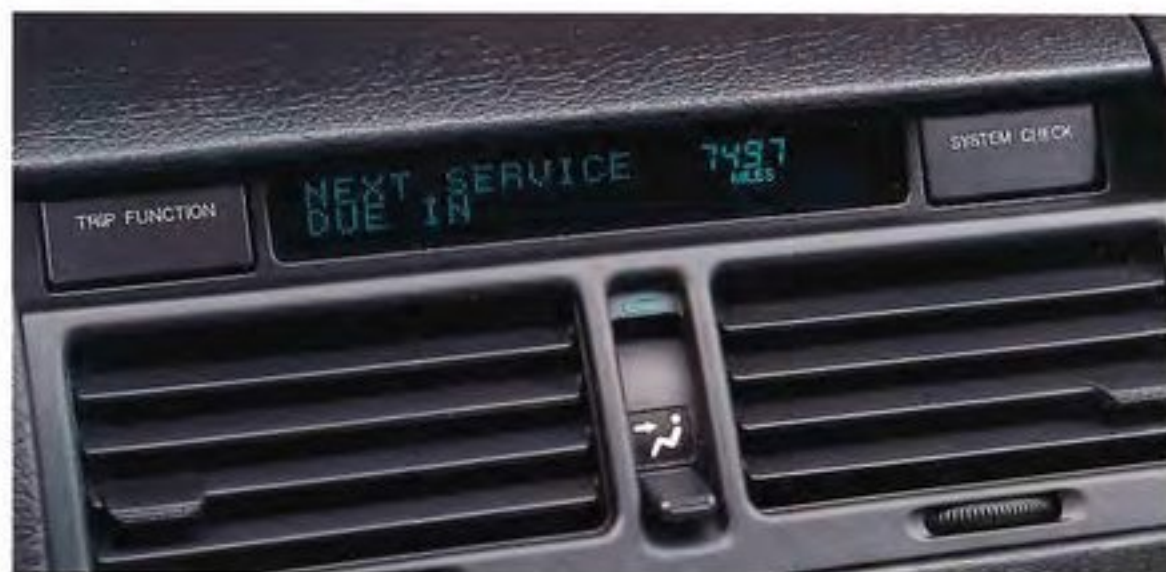
The Legend LS Driver's Information Center displays oil, coolant and washer fluid levels, time, distance traveled, fuel economy, mileage to next regularly scheduled service and mileage to empty.
