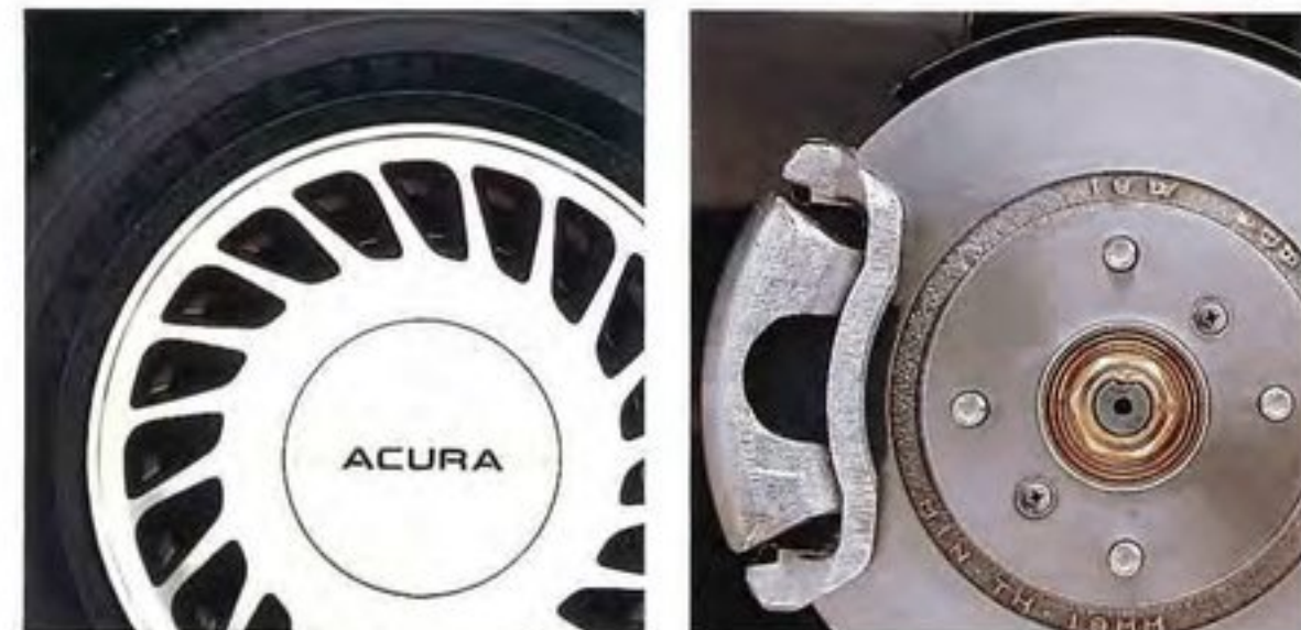
The Legend includes Michelin performance tires, alloy wheels and power-assisted four-wheel disc brakes. In addition, L and LS models feature an Anti-Lock Braking (ALB) system.
