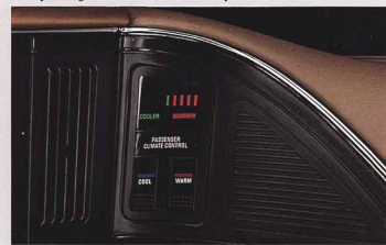
Front-passenger door controls for dual automatic ComforTemp climate control.
