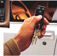
Available remote keyless entry system locks, unlocks doors, turns on interior lights, unlatches trunk, all from a distance.
