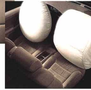
Driver and right front passenger air bags, used with three-point safety belts, can help prevent injury in certain frontal impacts of 14 mph or greater.
