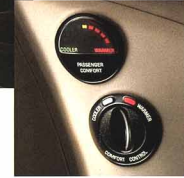
Dual automatic ComfortTemp climate control varies the temperature for driver and front-seat passenger.
