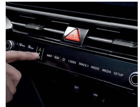
Infotainment/climate switchable controller share the same LCD softkey keyboard*
