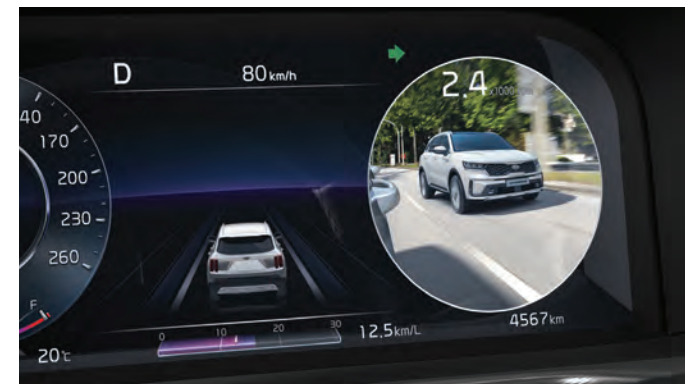
Blind view monitor displays the blind spot in the direction your turn signal is indicating.*
