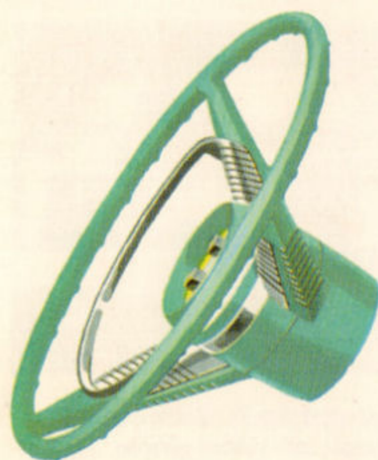
SAFETY STEERING WHEEL —Inverted center is designed to distribute stress under impact. Rubber-padded hub ring further protects the driver.
