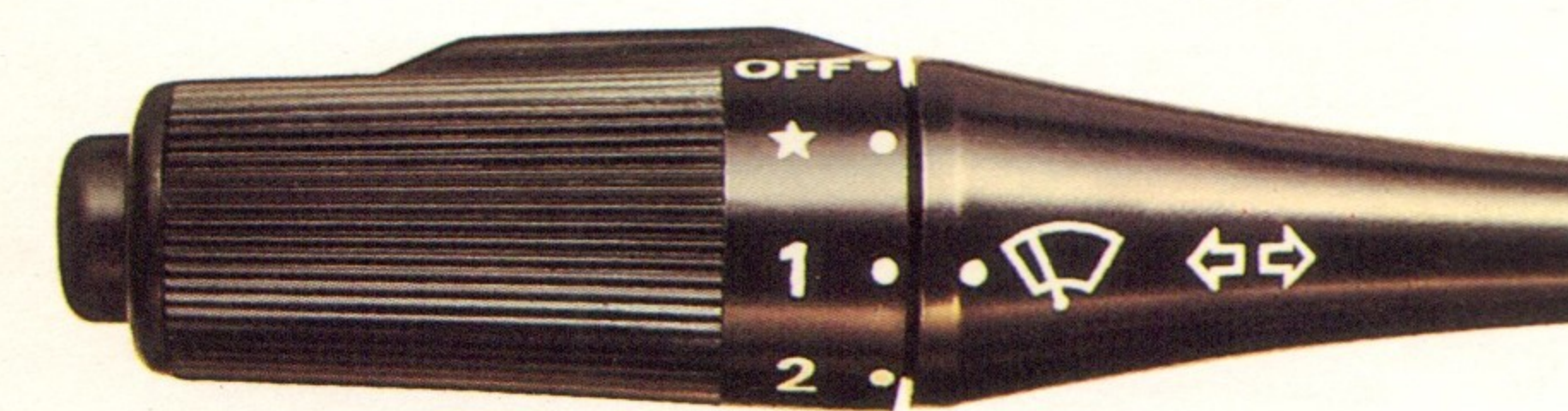
Variable intermittent wipers can be set at intervals from 3 to 12 seconds.
