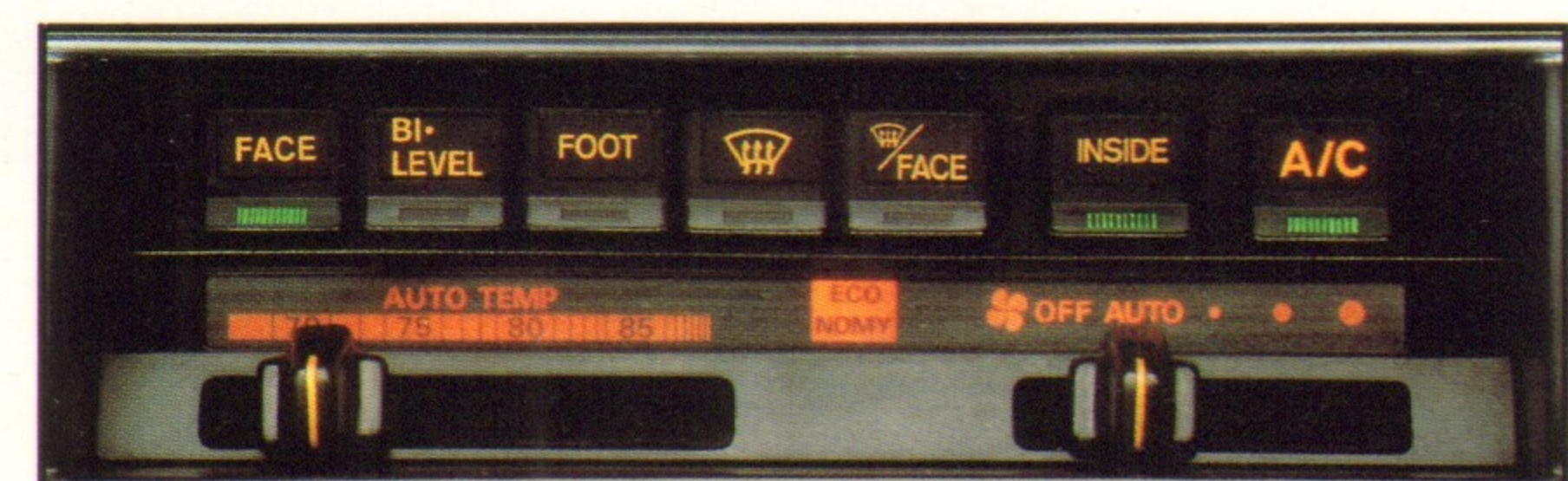
Automatic temperature control air conditioning and dual bi-level heating/ventilation allow you total environmental control.
