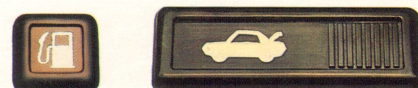
Starion offers the convenience of remote hatch and locking fuel lid releases.
