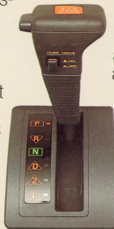
The smooth four-speed automatic overdrive ELC™ transmission has electronic operation and handy overdrive lockout switch.
