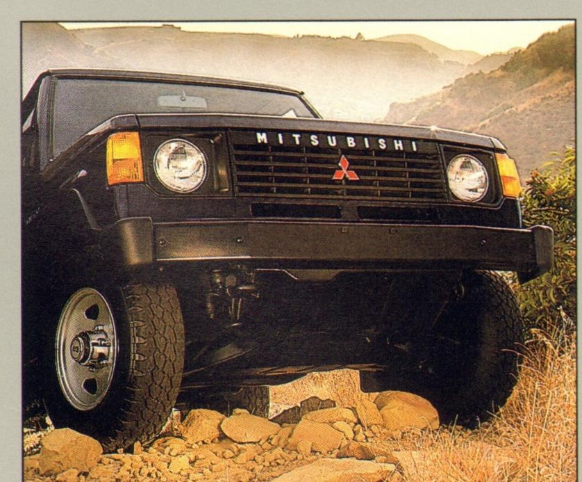
TAKING THE HIGH ROAD Montero's front differential is mounted directly to the frame providing a full 9.1 inches of ground clearance, with 8.3 inches minimum running ground clearance at the rear differential.
