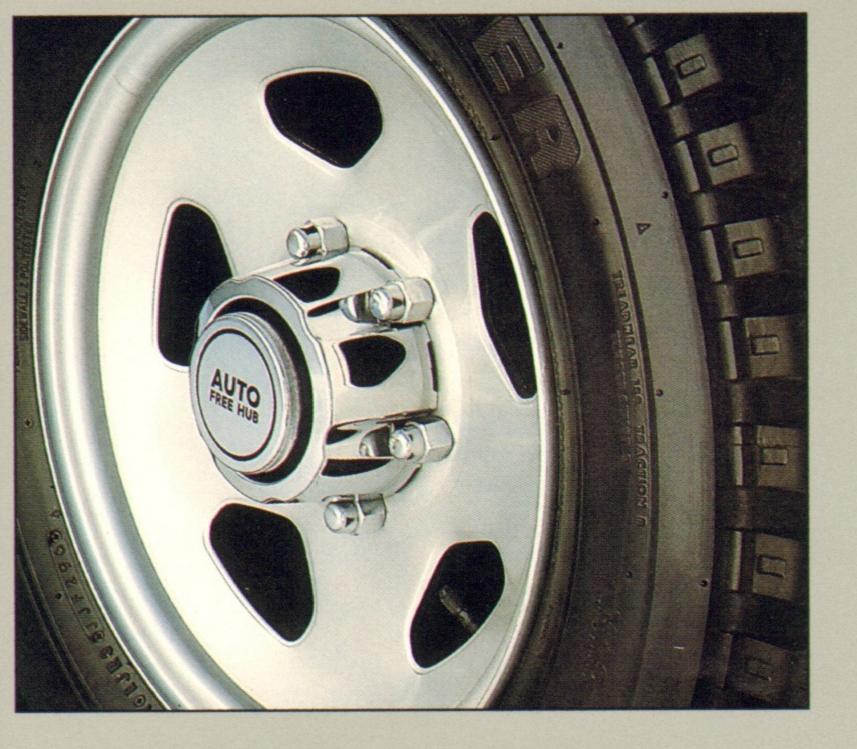
THE CONVENIENCE OF AUTO-MATIC HUBS Automatic locking front hubs are an important feature of the SP package. They allow the driver to shift from 2-wheel to 4-wheel drive without leaving the cab.
