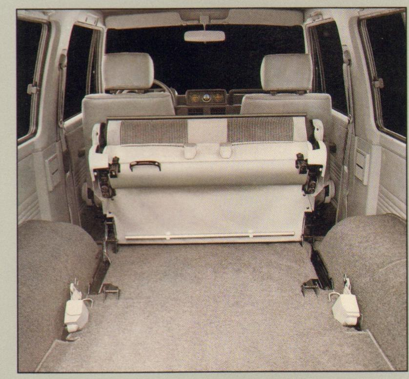
THE CONVENIENCE OF SPACE The Montero offers an optional rear seat that folds down to leave room for extra cargo or can be removed to give you 62.9 cubic feet of cargo capacity.
