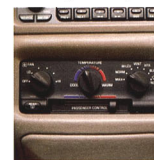
Available dual-zone ComfortTemp climate control option allows driver and passenger to vary each separate temperature.
