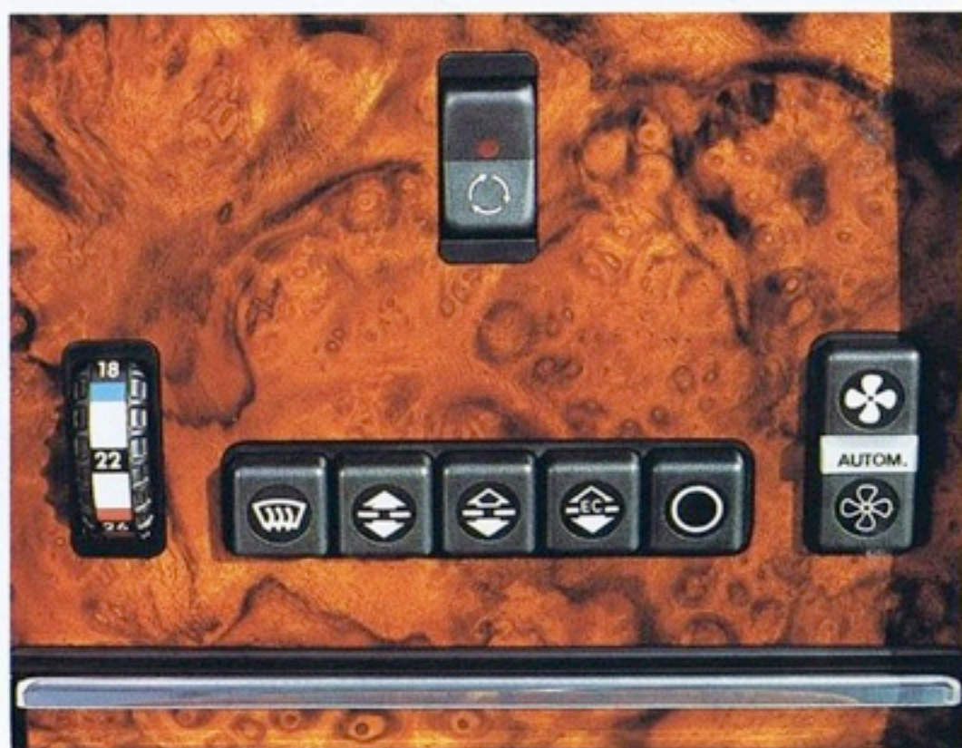
Automatic climate control. For electronic regulation of the temperature inside the car.
