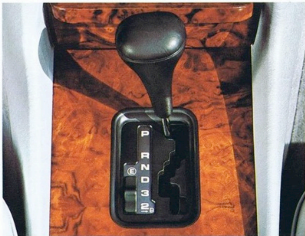
Automatic transmission saves you the trouble of declutching and changing gear, and offers you a choice of two shift programmes, Standard and Economy.
